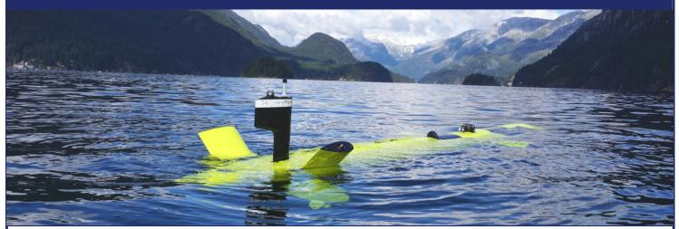
The Explorer class of AUV is a modular vehicle comprising of a forward free-flooding section, full diameter pressure hull and a free flooding aft section. It is optimized for longevity and can be adapted to meet new requirements. It is available in many configurations and depth ratings from 300 m to 6000 m.
