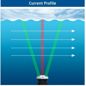
The AWAC uses the three slanted beams to measure the current profile over a range determined by the acoustic frequency. Large transducers transmit narrow acoustic beams and provide accurate data. The AWAC will alternate between wave data collection and current profiling. If the wave data collection is longer than the interval between current profiles, the AWAC will skip a current profile to ensure continuous wave data. Please contact Nortek if concurrent wave and current information is required.
